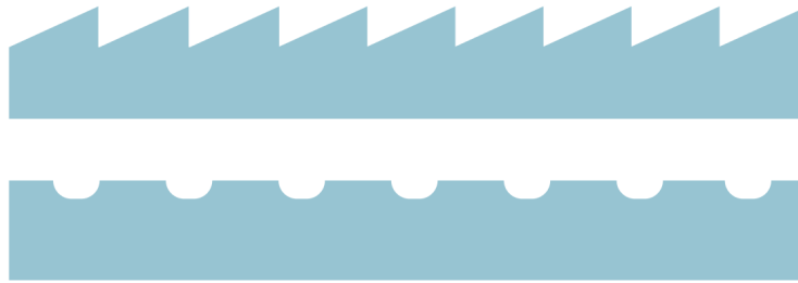
Figure 9: The groove profile of a ruled diffraction grating (above) and a holographic diffraction grating (below).
